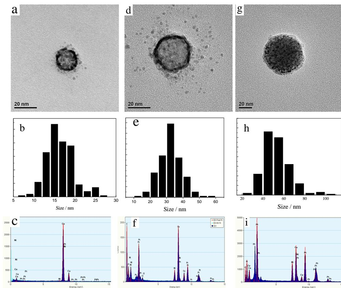
Fig. 4-9 TEM images, size histogram and EDX patterns of NiPt nanoparticles obtained at different temperatures. (a, b, c) 0 °C; (d, e, f) 25 °C; (g, h, i) 60 °C
