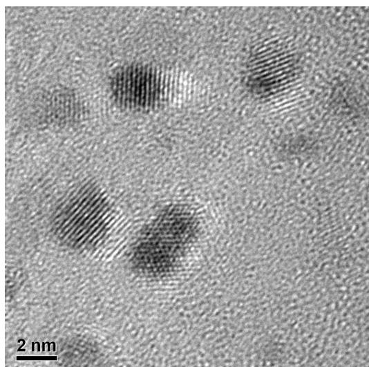
Fig. 4-8 HRTEM image of small nanoparticles around NiPt nanoparticles
