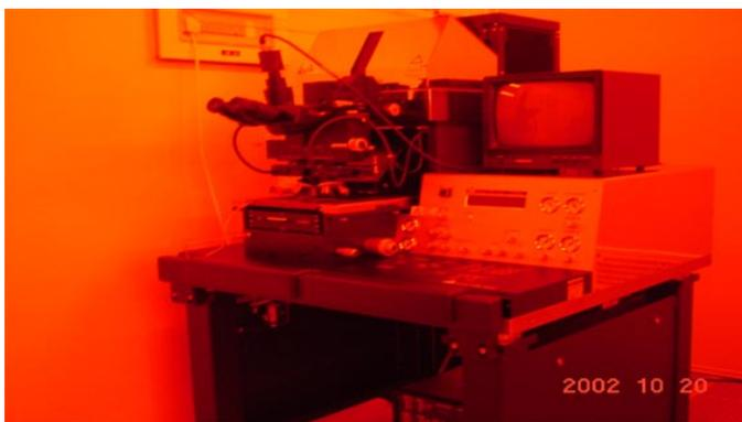
**Fig. 2-6 Digital photography of the Bonding Alignment Lithography machine (Karlsuss MA6/BA6, made in Germany)**
