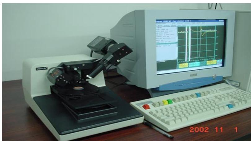
Fig. 2-8 Photo of the instrument of thickness measuring (Dektak3 Series)
