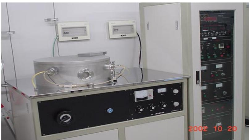
**Fig. 2-7 Digital photograph of the instrument of magnetron sputtering (JS-3X-100B, made in Beijing)**
