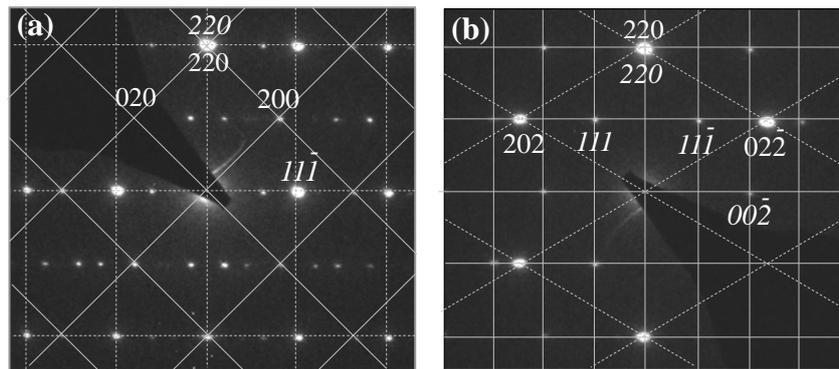
Fig. 5.4 (a), (b) Two typical SAED pattern of the Pd nanorod, demonstrating that the nanorod has a fivefold twinned structure.
